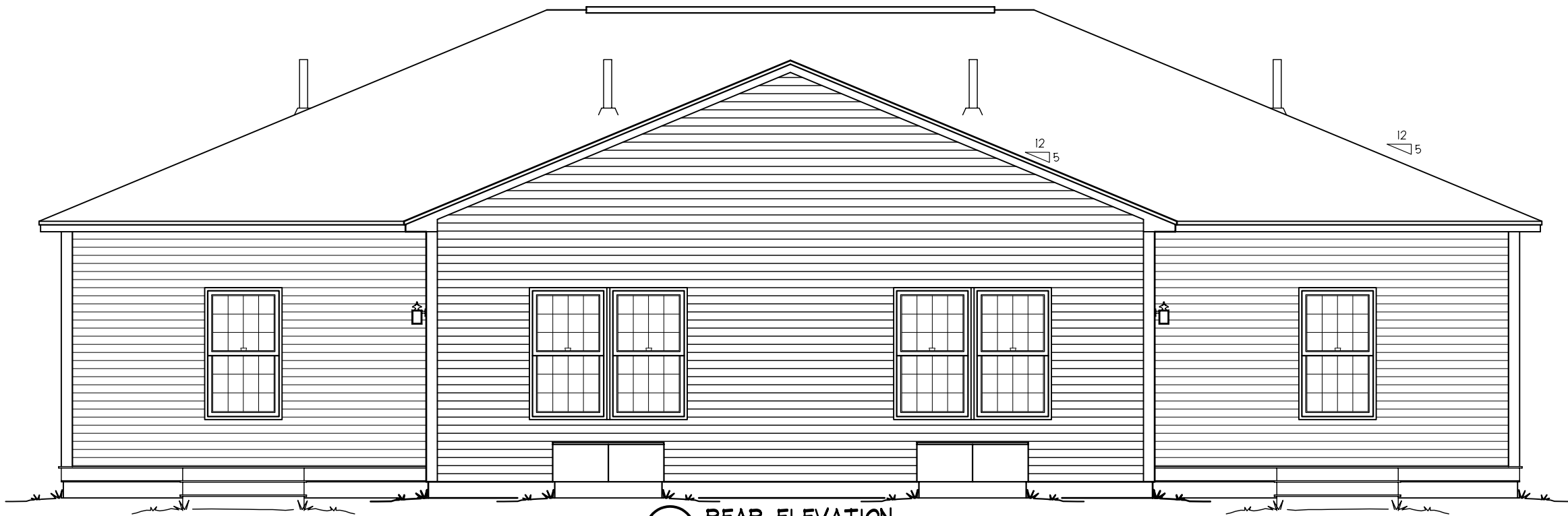
E-2 REAR ELEVATION SCALE: 3/16" = 1'-0"
